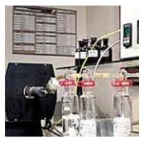
materials from cables- Part 2-1: Procedures. Determination of the amount of halogen acid gas.
